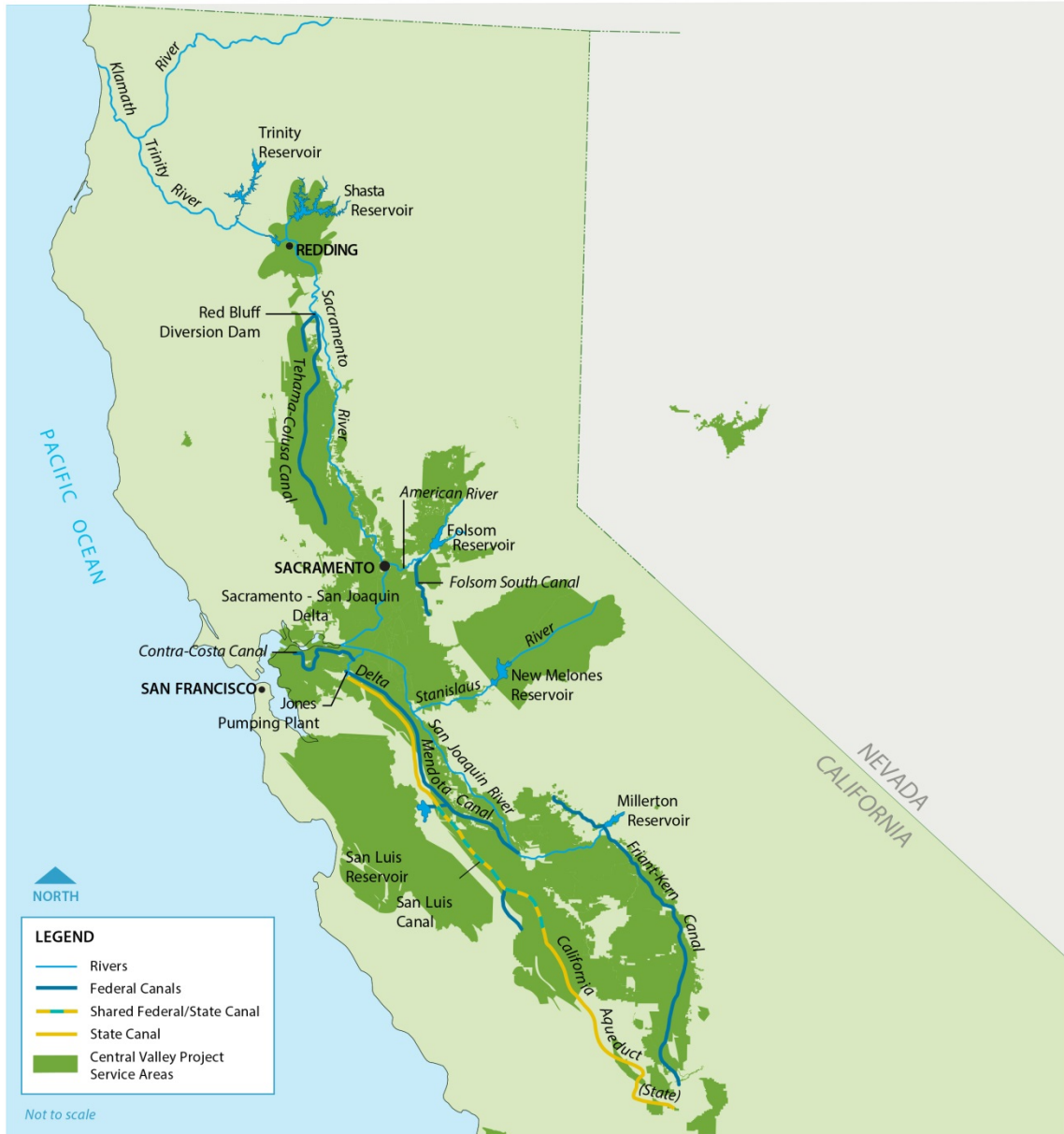
Figure 1-1. Major CVP Facilities and CVP Service Areas
